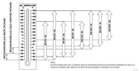
Figure 41. Engine Oil Operating Temperature Specifications - Deutz 2011
