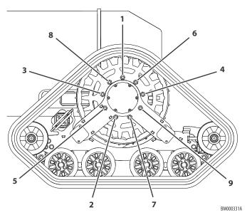
Figure 32. Quad Track Torque Sequence
