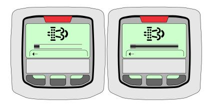
After the cleaning process is complete, the engine will run for approximately 5 minutes to allow the engine and Exhaust After Treatment (EAT) to cool down. The Indicator Gauge will display the "Regen Complete" screen as shown and the Emissions Temperature indicator will no longer be illuminated.
