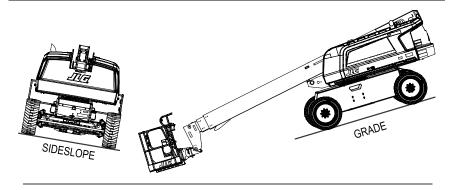
LEVEL Figure 14. Grade and Side Slope
