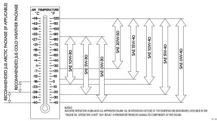
Figure 40. Engine Oil Operating Temperature Specifications - Deutz 2.9L
