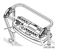
Operator passes through path of sensor beam.
