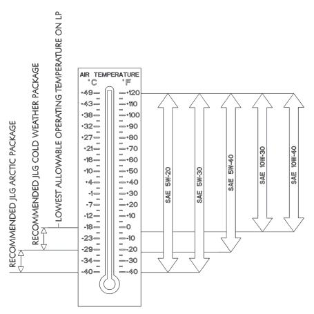
Figure 42. Engine Oil Operating Temperature Specifications - Ford MSG425
