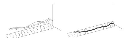
Figure 3. Parent Metal Crack
