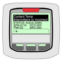
Figure 8. Engine Diagnostic Screen
