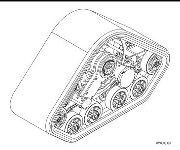
The Quad Track option consists of four track assemblies which are designed to be installed in place of the tire option.
