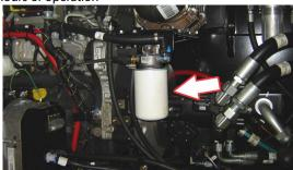
12. Fuel Pre-Filter - Deutz D2.9/TD2.9, 2.2L Stage V Lube Point(s) - Replaceable Element Interval - Drain water daily; Every year or 600 hours of operation
