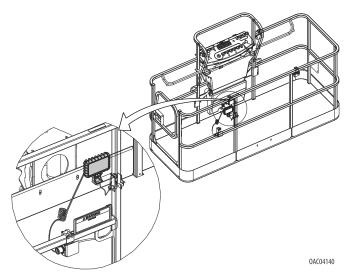
Figure 31. Portable Work Light
