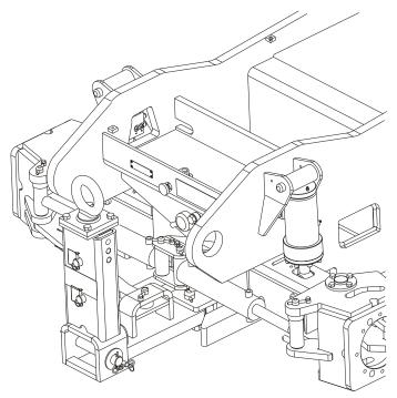
Figure 18. Towbar (Raised Position)
