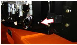
2. Swing Drive Hub Lube Point(s) - Level/Fill Plug Capacity - 32 oz. (0.95 L) Lube - 80w90 Gear Oil
